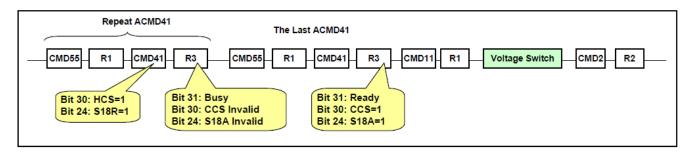
Figure 6-6-5 : ACMD41 Timing Followed by Voltage Switch Sequence
