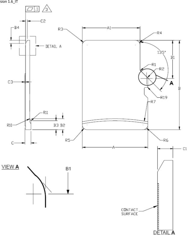
Figure 3-15-2: Dimensions Of microSD (Top View)
