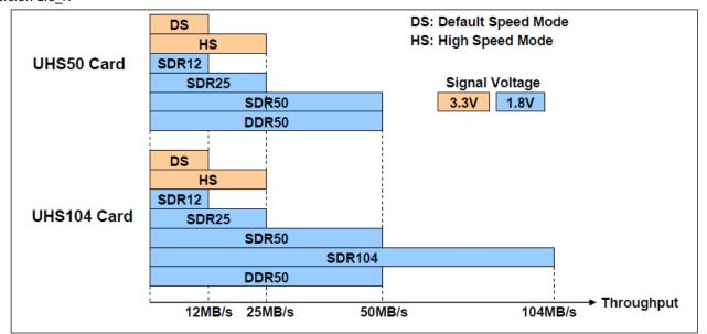
Figure 3-2-2 UHS-I Card Type Modes of Operation versus Throughout
