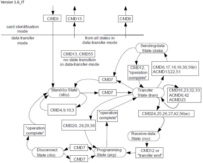
Figure 6-6-11: SD Memory Card State Diagram (data transfer mode)
