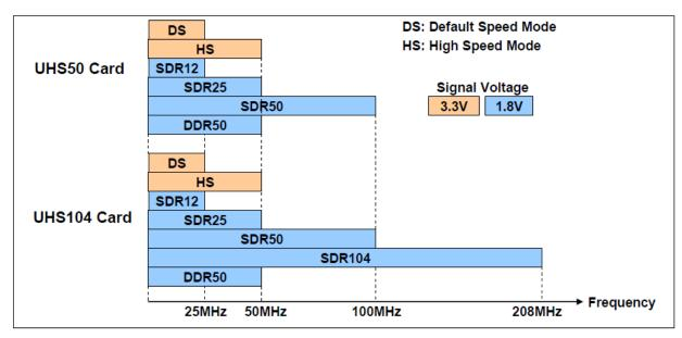
Figure 3-2-1 UHS-I Card Type Modes of Operation versus Frequency Range
