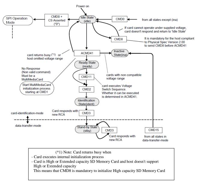
Figure 6-6-1: SD memory card diagram
