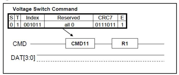
Figure 6-6-9 : Voltage Switch Command
