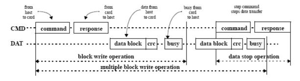
Figure 6-1-3: (Multiple) Block Write Operation
